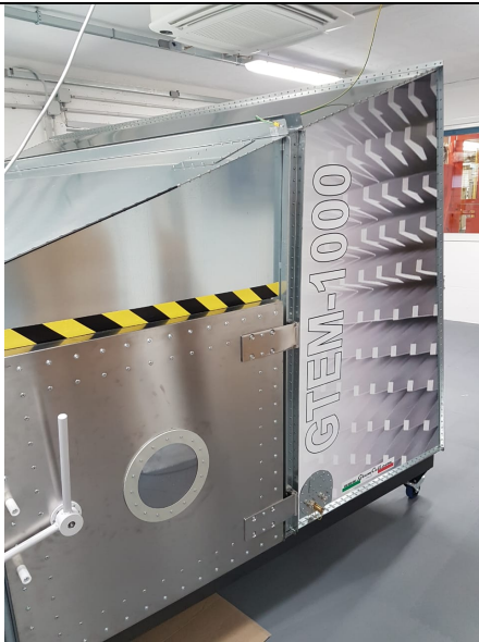
Special Multi-grip rivets system to join the metal sheets
