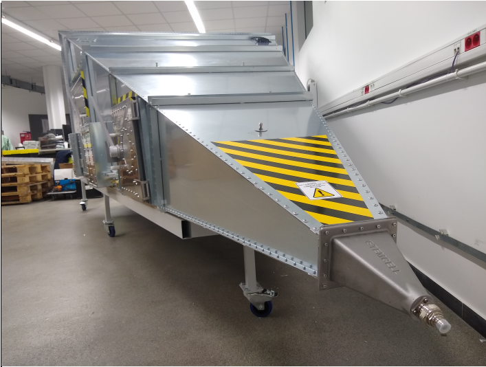
Unique Rectangular to coaxial flange transition to 7/16" connector + 7/16 to N or SMA transitions for microwaves
